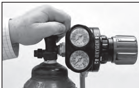
Figure 10: Opening the Cylinder Valve
