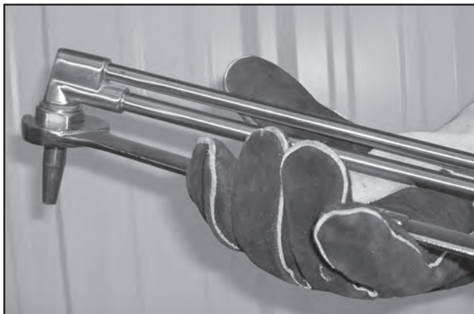
Figure 17: Tightening the Tip Nut
