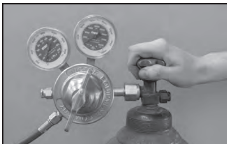
Figure 10: Opening the Cylinder Valve
