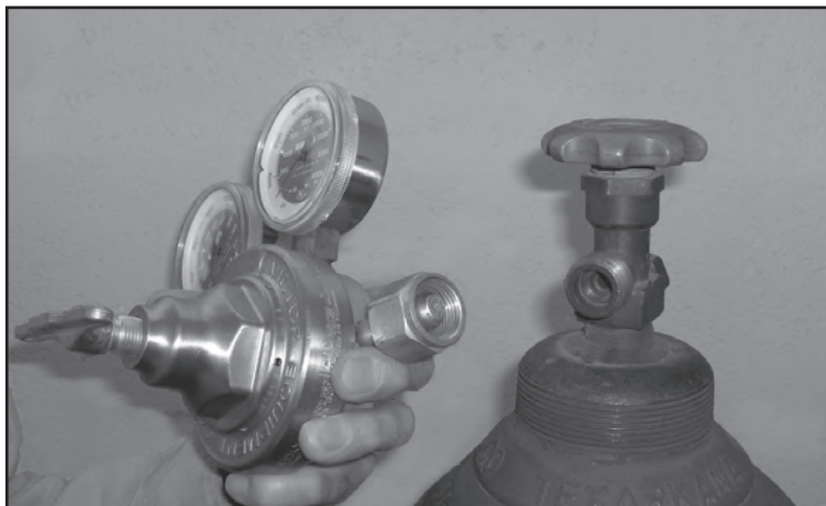
Figure 9: Inspecting the Cylinder and Cylinder Valve
